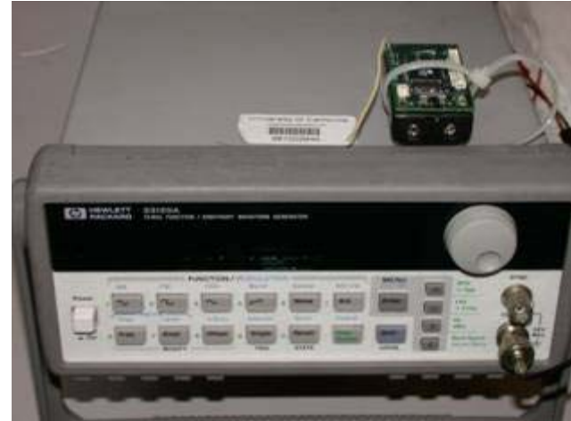
Fig2: Sensor node mounted on a function generator
